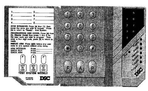
Zone Lights 1 to 8 indicate zone activity. With the system disarmed, the Zone Lights will come ON to indicate when zones are active, and the Zone Lights will be shut OFF to indicate that zones are secure.
